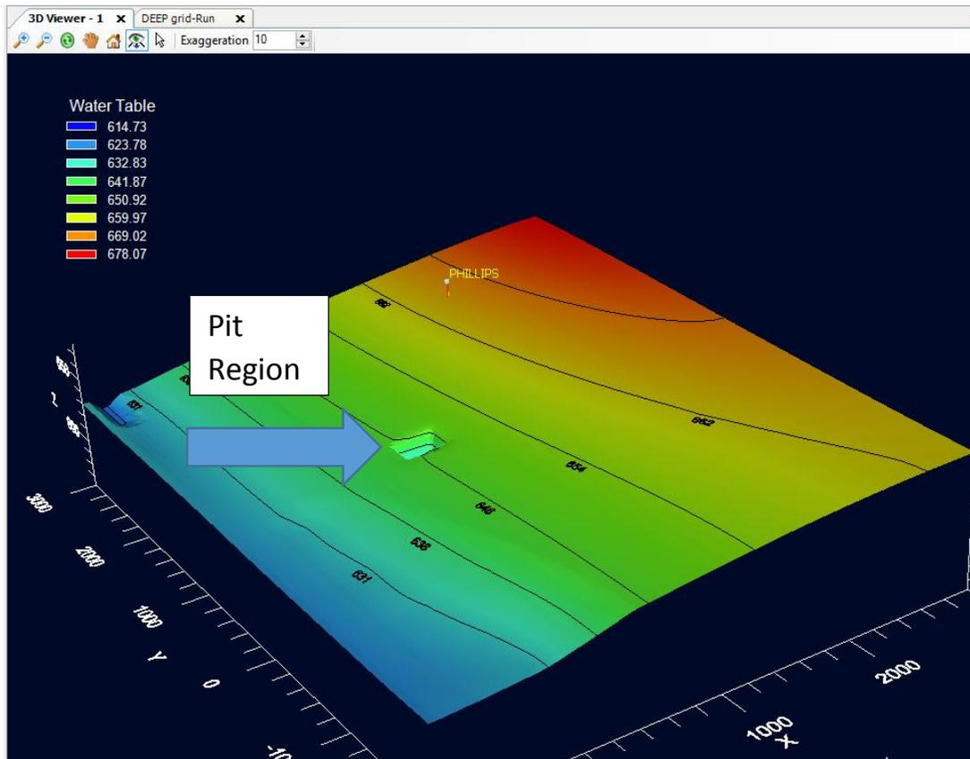
Figure 5: Water Table in 3D view; note the depression in the region of the pit
