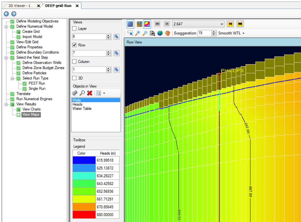
Figure 3 Water table in cross-section, over the well screen
