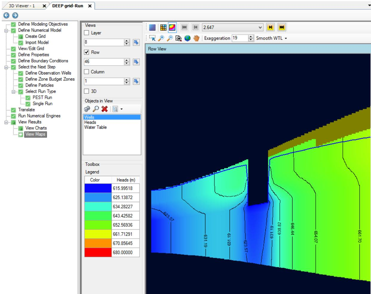
Figure 6: Cross-section through pit region showing water table
