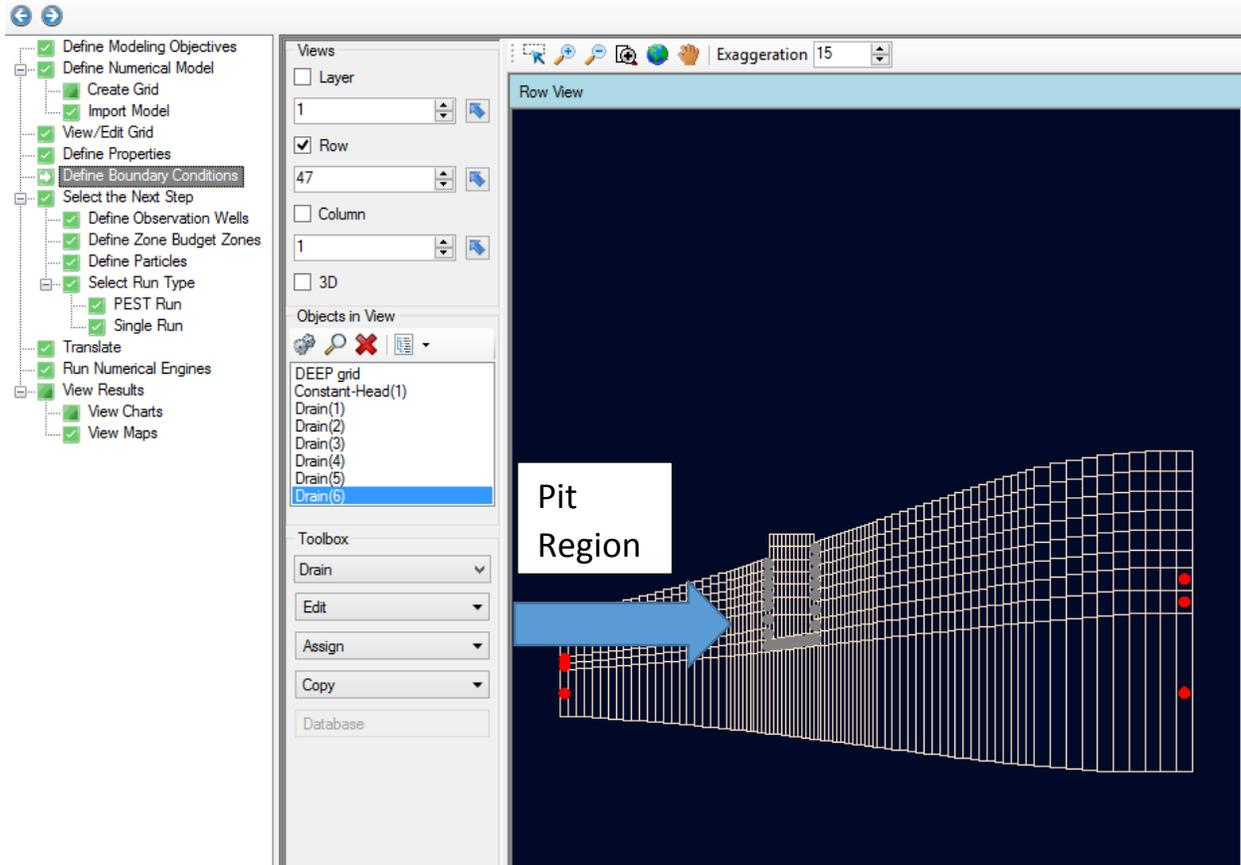
Figure 2: Cross-section view of pit region
