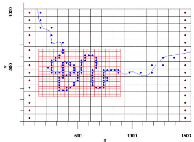
Figure 6: Numerical model equivalents; blue points are river cells, red are constant heads.
