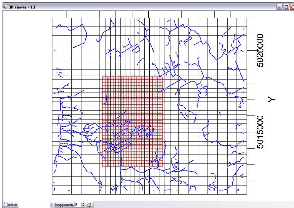
Figure 4: 2D Viewer showing parent grid (grey gridlines) and child grid (red grid lines) in Visual MODFLOW Flex
