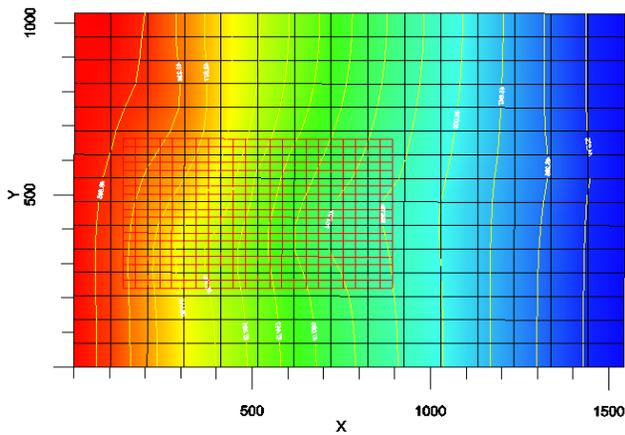
Figure 7: Combined parent and child grids heads with contours
